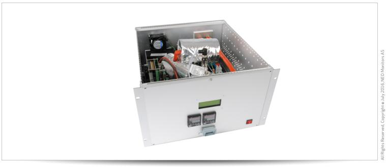
**NEO Monitors LaserGas™** is using Tuneable Laser Absorption Spectroscopy (TLAS) i.e. a non-contact optical measurement method employing solid-state laser sources. Therefore, the sensor remains unaffected by contaminants and corrosives and does not require regular maintenance. The laser beam is coupled into a measurement cell, where it is reflected one time from a flat mirror in order to enhance the analyzer sensitivity.
