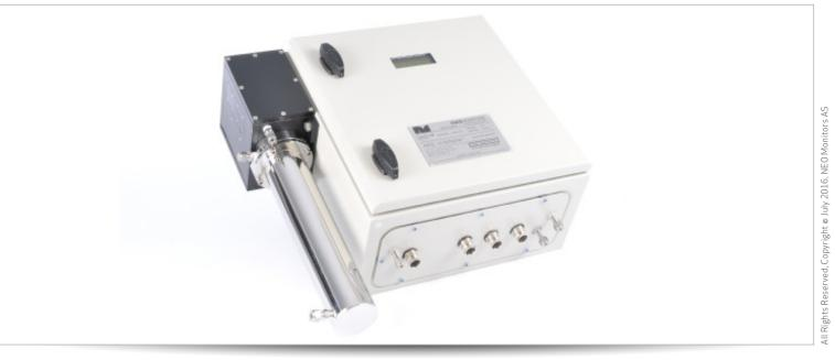
**NEO Monitors LaserGas™** is using Tuneable Laser Absorption Spectroscopy (TLAS) i.e. a non-contact optical measurement method employing solid-state laser sources. Therefore, the sensor remains unaffected by contaminants and corrosives and does not require regular maintenance. The laser beam is coupled into a Herriott cell, where it is reflected multiple times between two spherical mirrors in order to enhance the analyser sensitivity.
