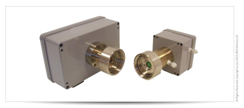
**NEO Monitors LaserGas™** is using Tuneable Laser Absorption Spectroscopy (TLAS) i.e a non-contact optical measurement method employing solid-state laser sources. The sensor remains unaffected by contaminants and corrosives and does not require regular maintenance. The absence of extractive conditioning systems further improves availability of the
